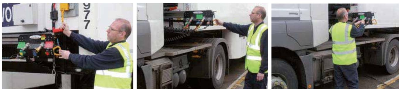
Pulling down on RED Locking Handle and drawing the YELLOW Handle outwards allows the noseplate to extend beyond the edge of the trailer.
